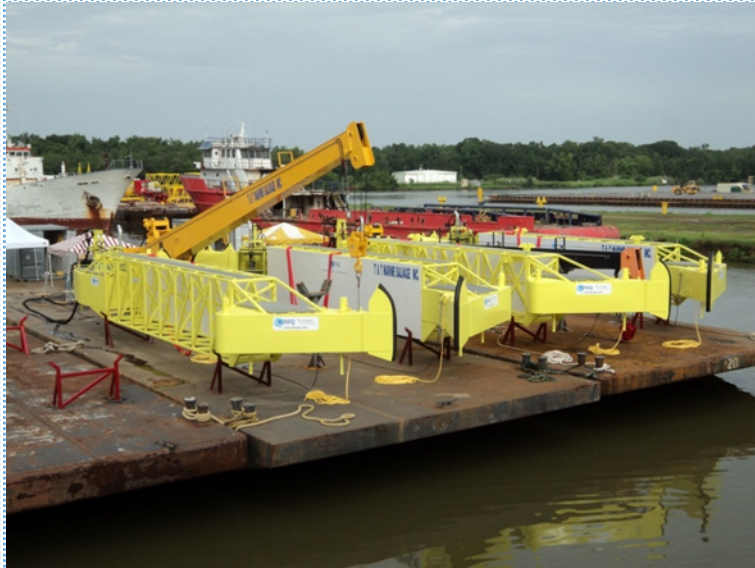
Barges utilized for near shore skimming
